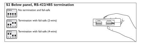
Note! DIP-switch alterations are only effective after a power on.
