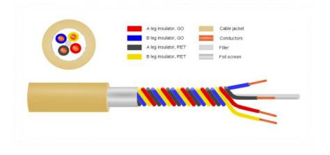
In the above, cable Red - Blue are joined and Black – Yellow are joined. The tight winding around the central filler gives the cable its exception noise immunity characteristic. When, making the cable off, it is important to keep the conductors the same length and keep the unwound length to a minimum.
